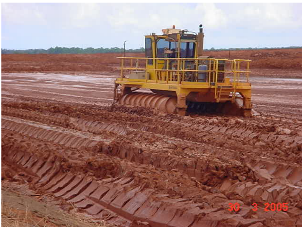
Figure 1.5 The operation of an Amphi-roller on the Residue
