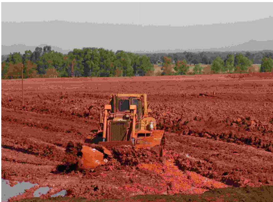
Figure 1.6 Operation of dozer on “wet” residue
