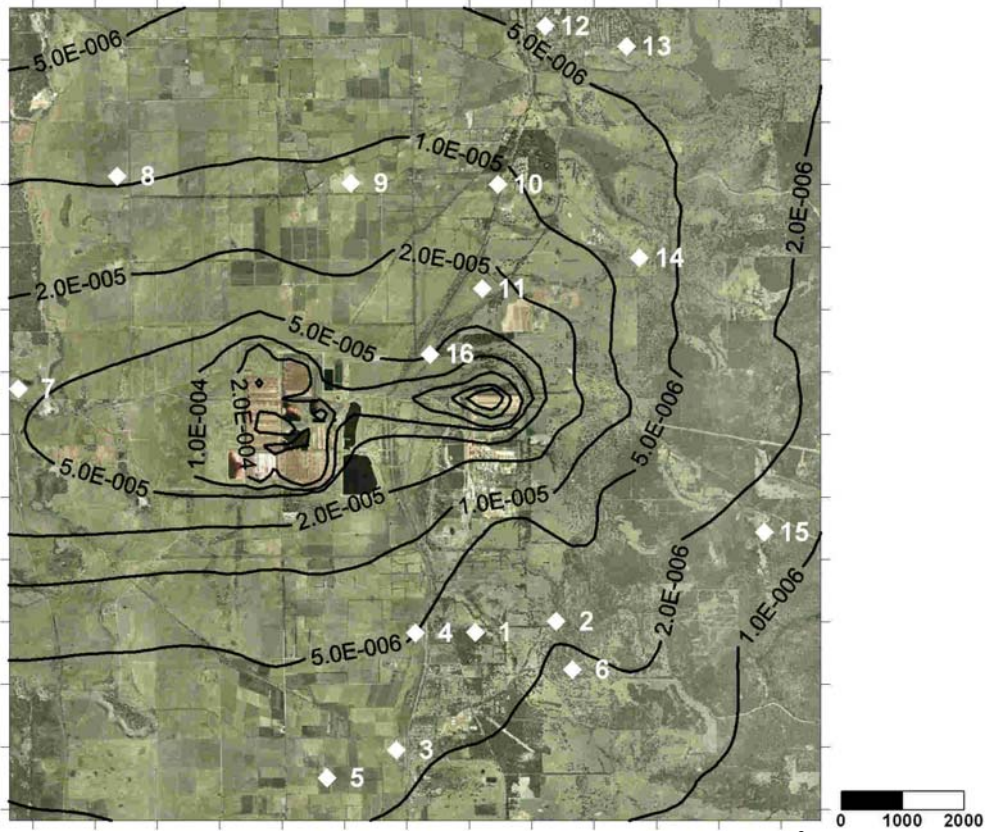
Figure 8.4 Predicted Annual Average Arsenic Concentrations ( \mu\text{g}/\text{m}^3 ) from the Base Case Refinery
