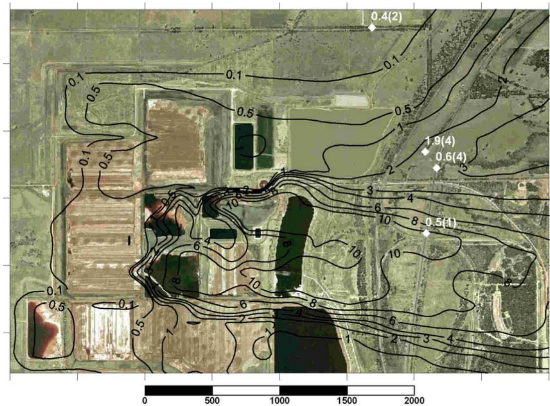
Figure 7.11 Predicted and Observed 1-hour Odour Levels (ou) for the hour ending 2200 WST on 26 February 2005
