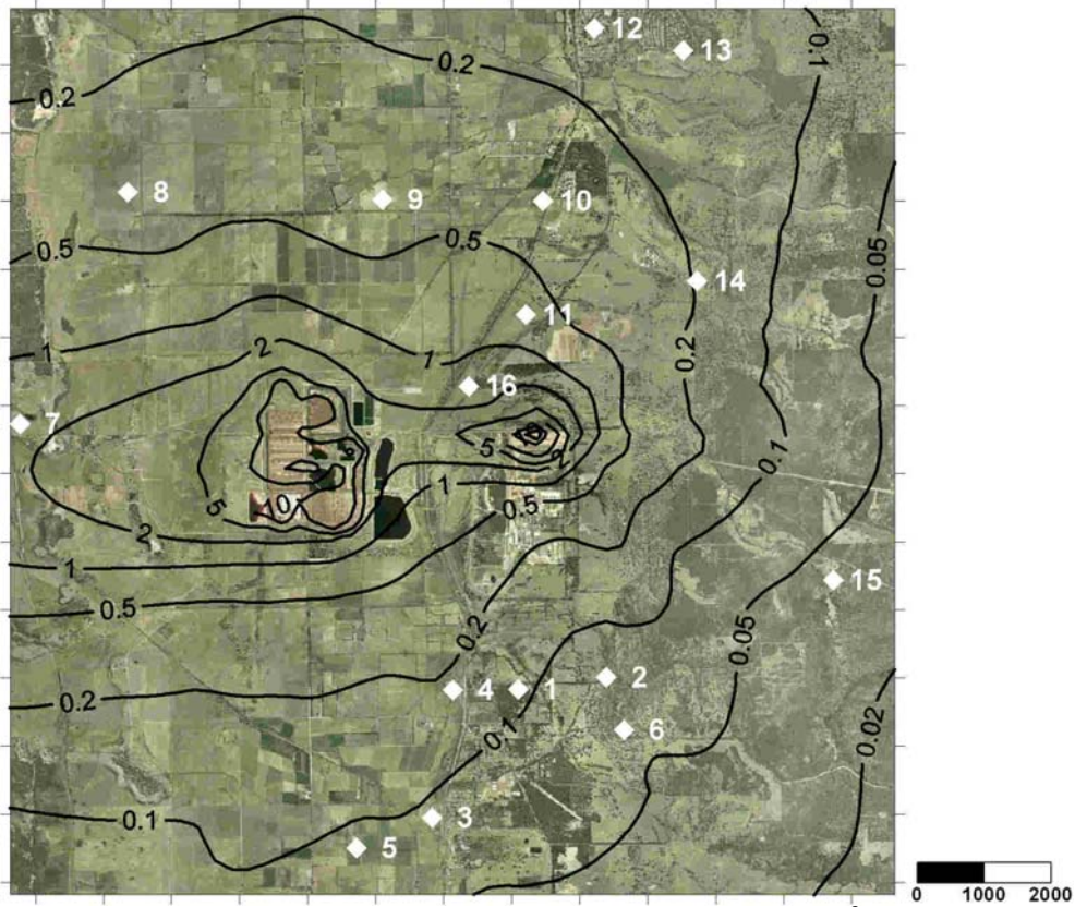
Figure 8.10 Predicted Annual Average PM 10 Concentrations (µg/m 3 ) from the Expanded Refinery
